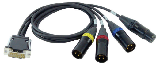
Breakout cable for Mini-DA42: input: 1 × AES42/AES3, output: 1 × AES3, 2 × analog
